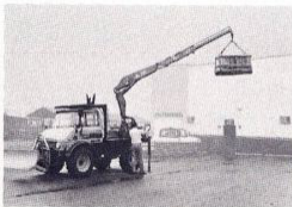
Sickle-bar, flail and rotary mowers are available for maintenance of industrial properties. A side-boom mower is shown for mowing slopes or rail right of way.
