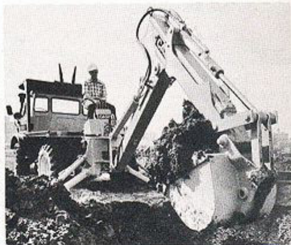
Four-wheel drive loader backhoe with dig depths to 15' (4572 mm).
