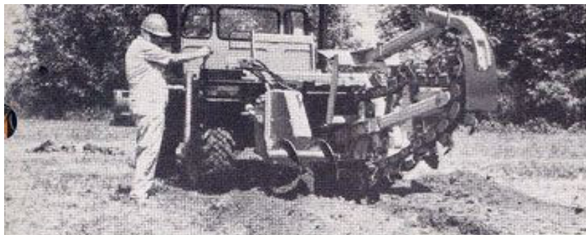
der trencher. Booms are available offering 7 different combinations of dig depth and trenching h. Hydraulic system controls raising, lowering.
