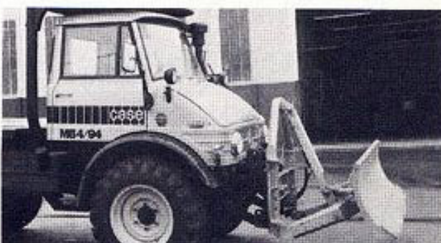
A backfill blade is a useful attachment for leveling unpaved supply yards and maintaining gravel roads and parking lots.
