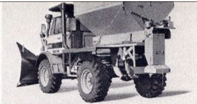
Snow and ice control is facilitated with this salt and sand or cinder spreader.
