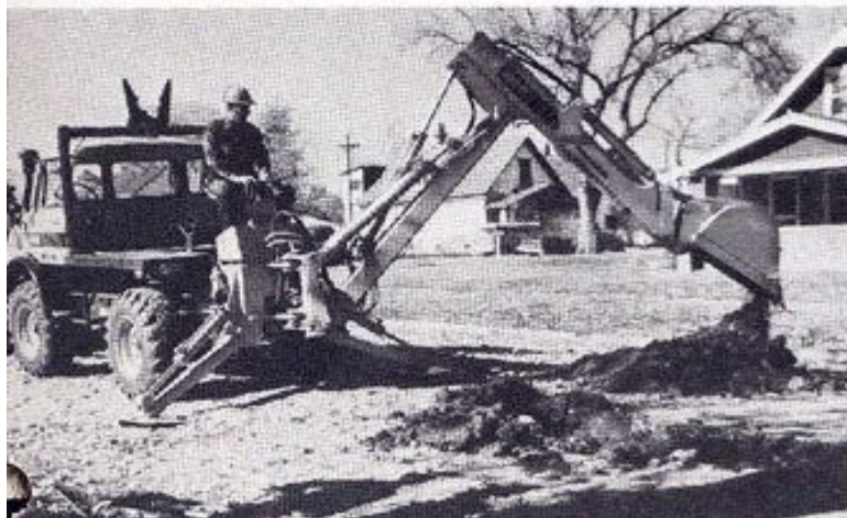
Case offers utilities a choice of 12' backhoe for use with Unimog, or 12' to 15' Extendahoe with hydraulic telescoping dipper. Both feature 190° foot swing with hydraulic swing cushioning.
