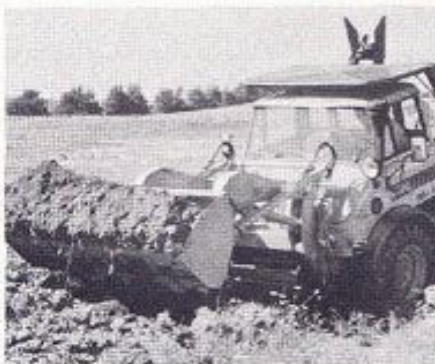
The \frac{3}{4} yd. 3 loader can be installed/removed in minutes. Self-standing when not attached. 2645-lb. lift capacity to 8'2" height.
