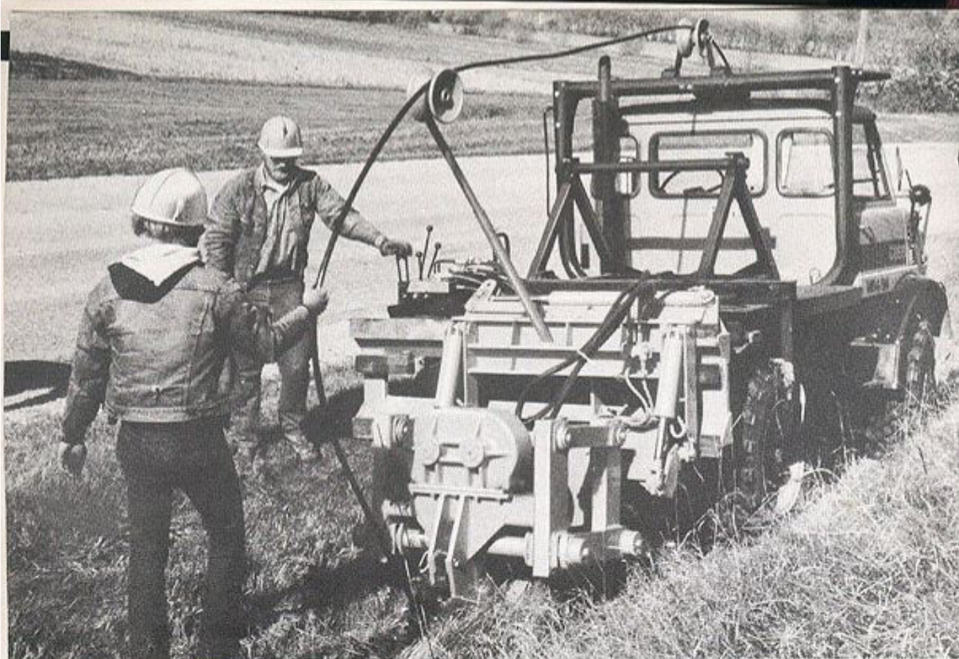
The Unimog can be a rear-mounted cable layer with vibratory blade for clean cutting action and minimal soil disturbance. Buries up to 2" O.D. cable to 30" cover depth. Also handles multiple size cable, tubing and hose.
