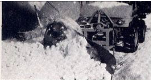
Unimog can be equipped with snow blower or snow blade for clearing plant yards and parking lots. Blowers and "V" plows are also available for use on tracks.
