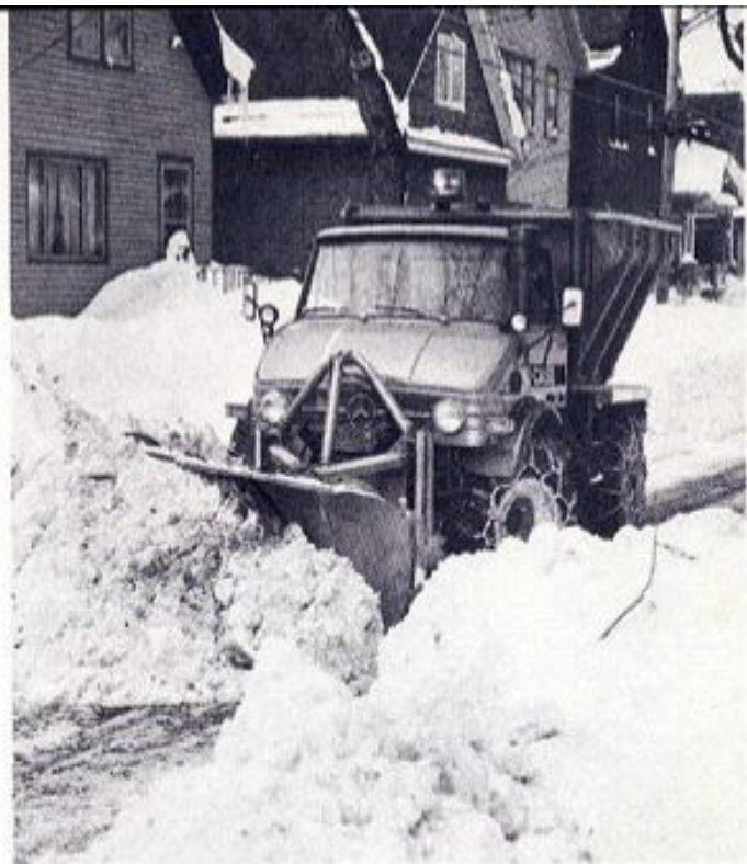
Snow fighting attachments for the Unimog include cutters, both single chute (cover photo) and double blowers, V-plows; spring-loaded blades; and salt/sand spreaders (shown on blade-mounted unit above). Photos here illustrate Unimog system at work in Buffalo, N.Y., clearing away record snowfalls of winter, 1976-77.
